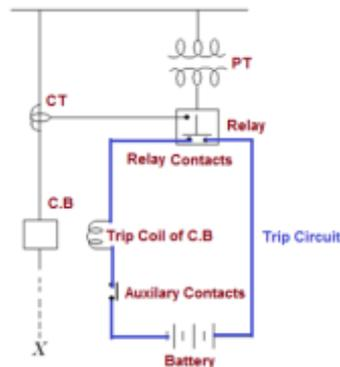
**Figure1. Working principle of relay**
