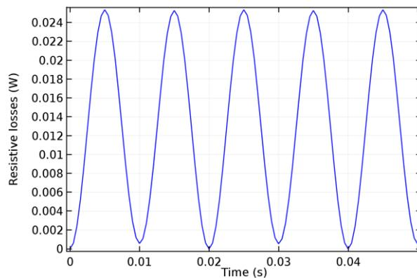
**Figure 6. Variation of resistive losses in windings with time for CNT**
