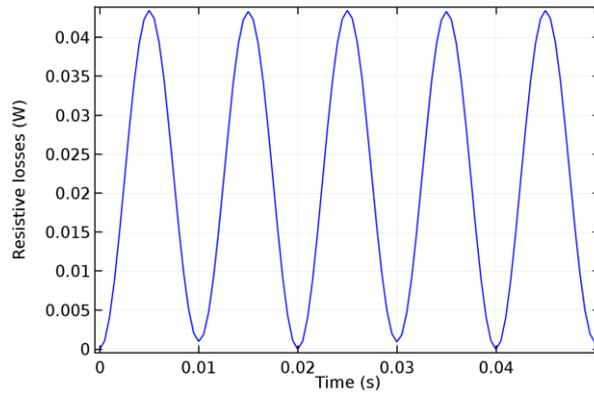
**Figure 5. Variation of resistive losses in windings with time for copper**
