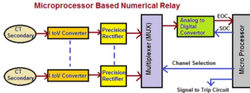
Figure4. Block Diagram of Numerical Relay
