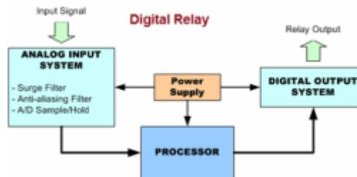
*Figure4. Block Diagram of Digital Relay*
