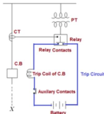
Figure1. Working principle of relay
