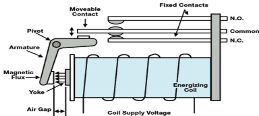
Figure2. Electromechanical Relay
