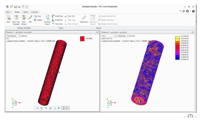
(Pipe increasing Temperature by the parabolic solar Concentrator at150C)
