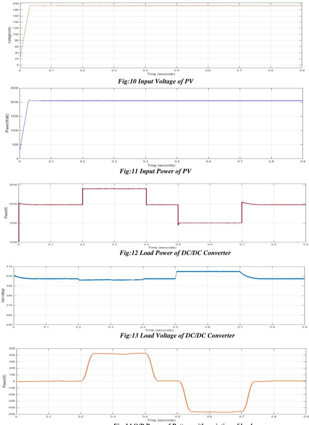
Fig:14 O/P Power of Battery with variation of load
