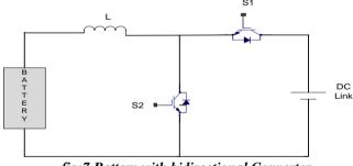
fig:7 Battery with bidirectional Converter
