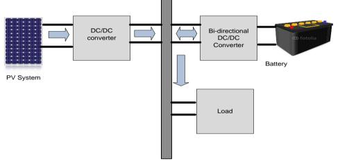
Fig 1:DC microgrid with storage system
