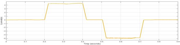
Fig:15 O/P Current of Battery with variation of load
