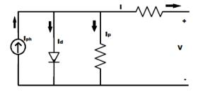
Fig: 2 equivalent circuit of PV cell
