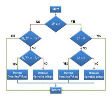
Fig: 6 Flow chart of incremental conductance
