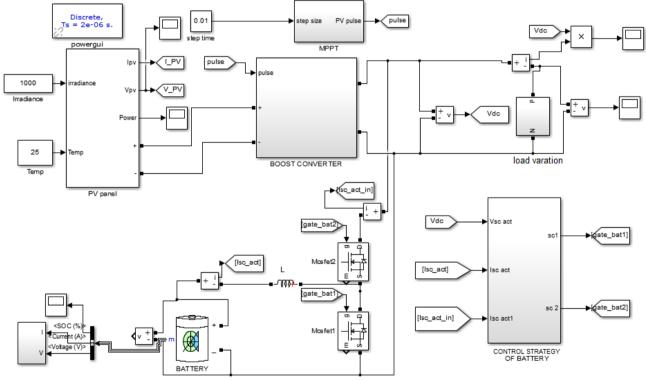
Fig:8 Simulation block of PV system with Battery
