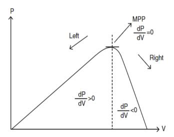
Fig: 5 P-V curve of incremental conductance method on a solar plane.
