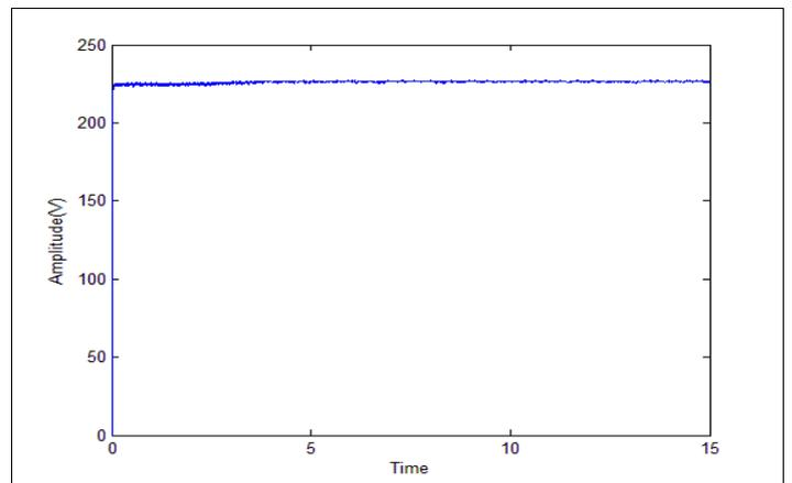
**Fig 8:- Output Voltage of Rectifier Unit**
