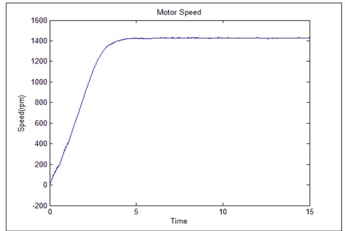
Fig 10:-Speed of Induction Motor
