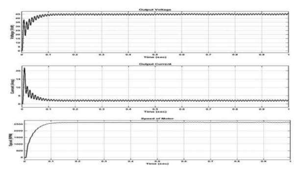
Fig.13 Waveform of o/p voltage, current and speed of the motor of Active front end converter
