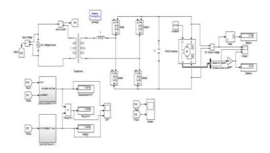
Fig.8 Simulation model of Diode Bridge front end converter
