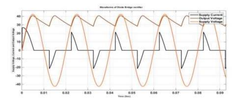
Fig. 2 Diode Bridge rectifier o/p voltage, current and i/p current waveform
