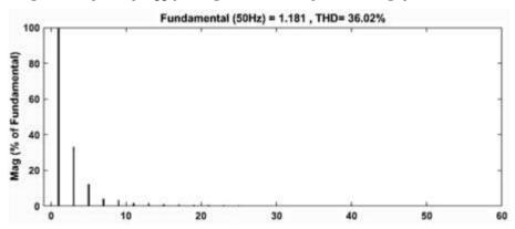
Fig.11 FFT analysis of supply side current
