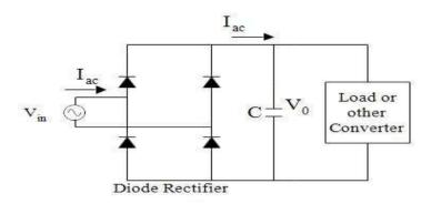
Fig.1 Diode Bridge rectifier with output capacitive filter
