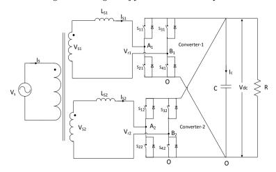
Fig.6 Circuit diagram of front end converter
