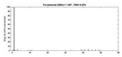
Fig.15 FFT analysis of supply side current
