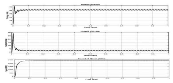
Fig.9 Waveform of o/p voltage, current and speed of the motor of Diode Bridge front end converter
