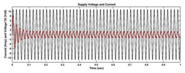
Fig.14 Waveform of supply voltage and current of Active front end converter
