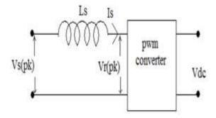
Fig.7 General Circuit diagram of PWM rectifier
