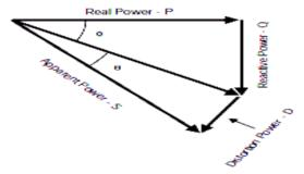
Fig.4 Power triangle for non-linear system
