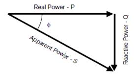
Fig.3 Power triangle for linear system
