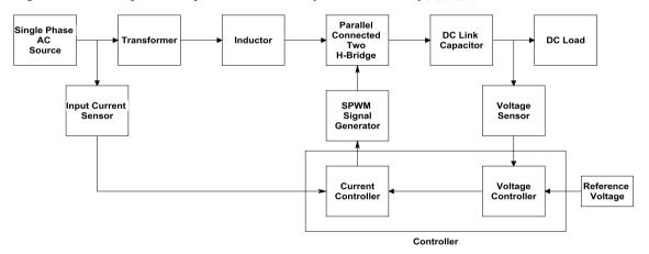
Fig.5 Block diagram of front end converter system
