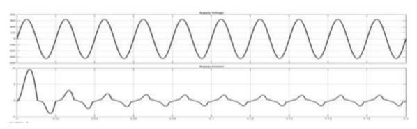
Fig.10 Waveform of supply voltage and current of Diode Bridge front end converter
