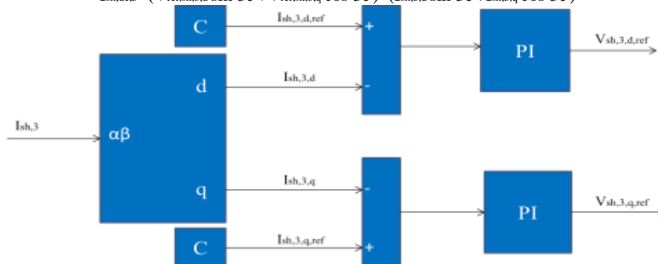
Fig. 4.5: Current controller block
