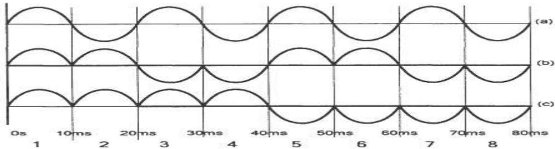
Figure 4 a) Input 50Hz (b) Output 25Hz
