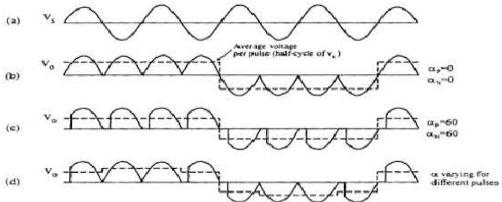
Figure 3 Single Phase Cycloconverter Outputs a) Input voltage b) Output voltage for zero firing angle c) Output voltage for firing angle of 60 degrees d) Output voltage with varying firing angle.
