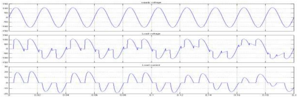
Figure 9 Waveform for the input frequency 2 times the output frequency
