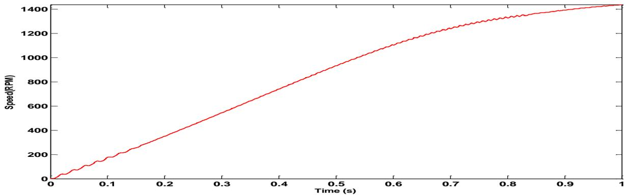
Figure 8 Speed Vs Time output of single phase induction motor at  $f=50$  Hz
