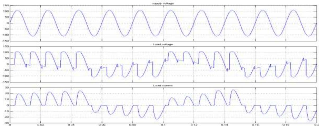
Figure 13 Waveform shows the input frequency is 5 times the output frequency
