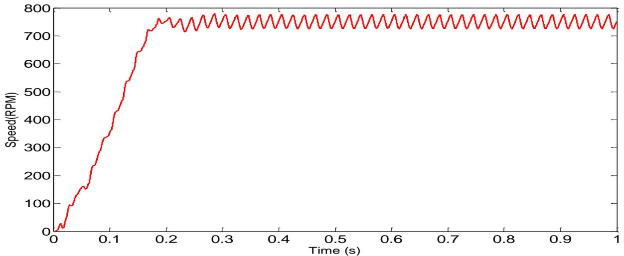
Figure 10 Speed Vs time output of single phase induction motor at  $f=25$  Hz
