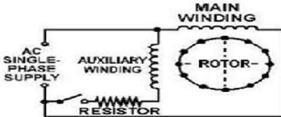
Figure 5 Starting circuit of 1- $\phi$  induction motor
