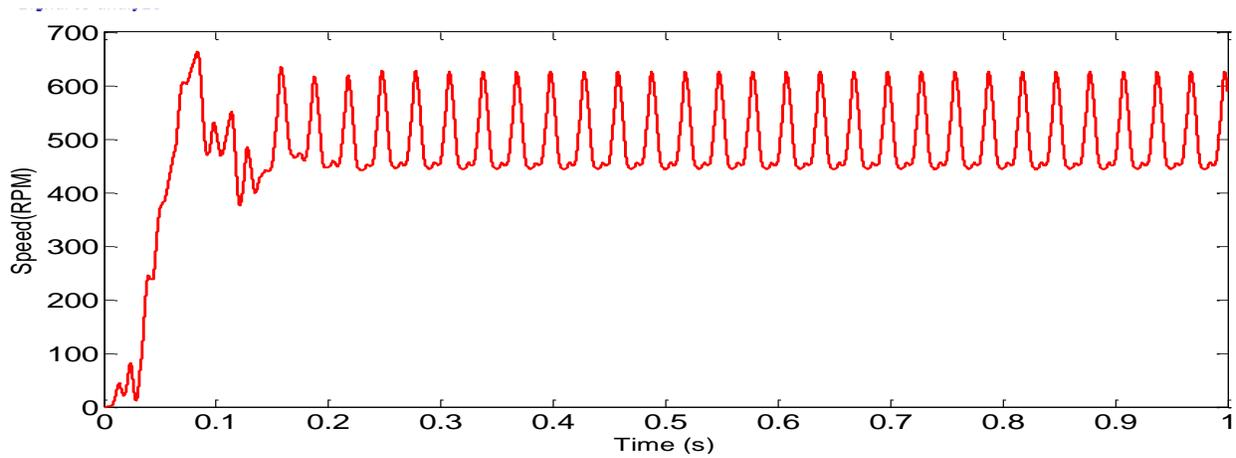
Figure 12 Speed Vs time output of single phase induction motor at  $f=16.66$  Hz
