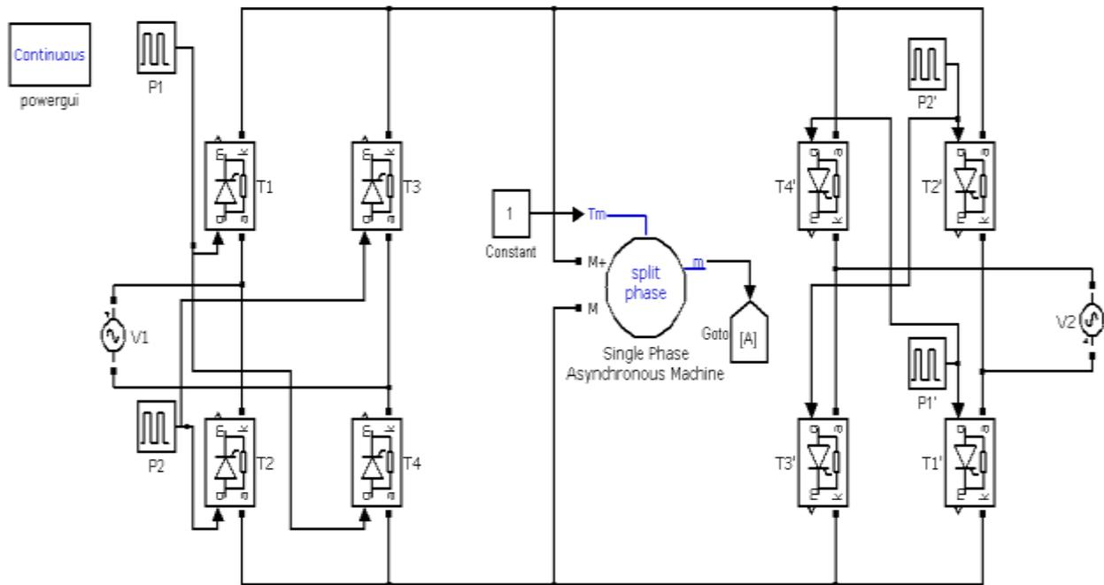
Figure 7 single phase cycloconverter model with single phase induction motor
