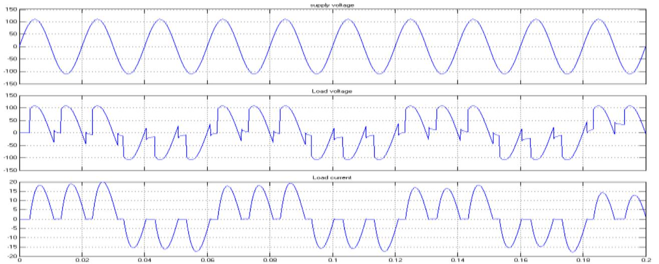
Figure 11 Waveform shows the input frequency is 3 times the output frequency
