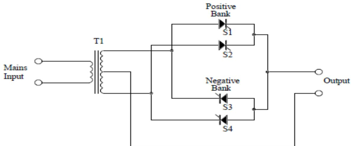
Figure 2 BASIC SINGLE PHASE CYCLOCONVERTER
