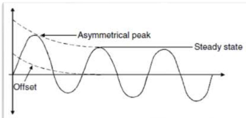
**Figure 1: Symmetrical and Asymmetrical Faults**
