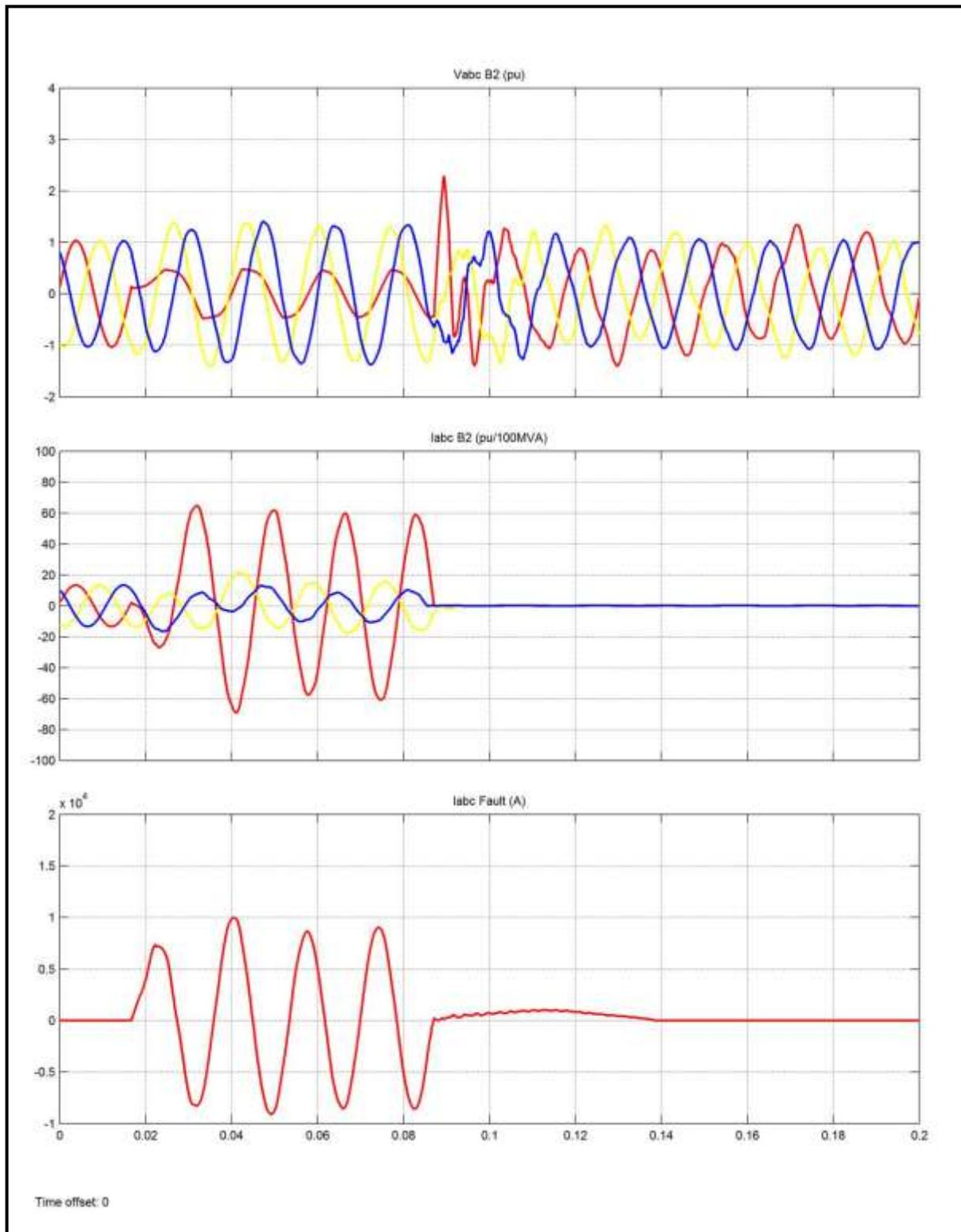
**Three phase permanent fault waveforms**
