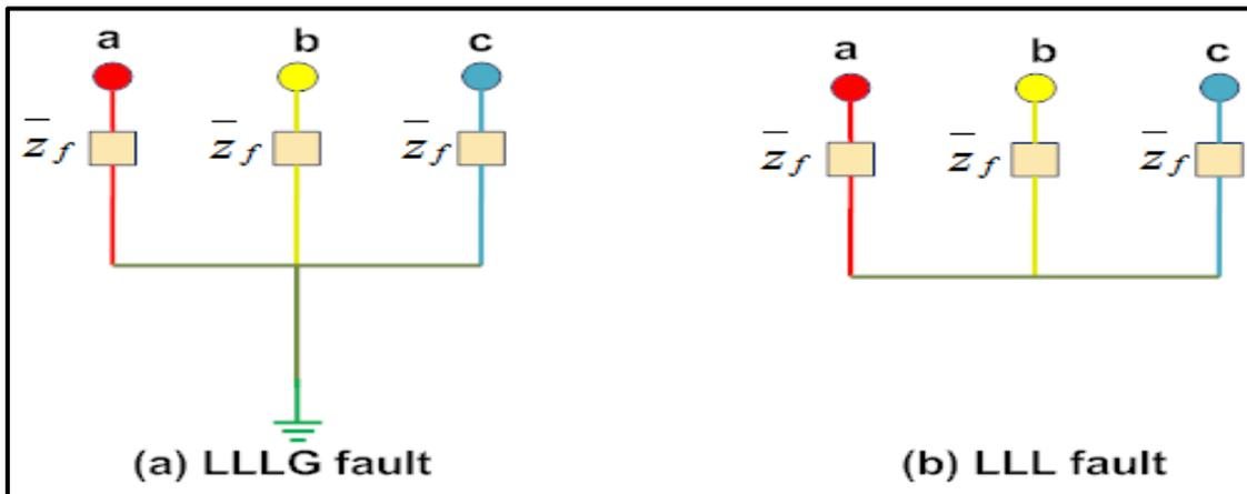
**Figure 2: Symmetrical faults**
