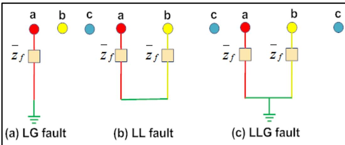
**Figure 3: Unsymmetrical faults**
