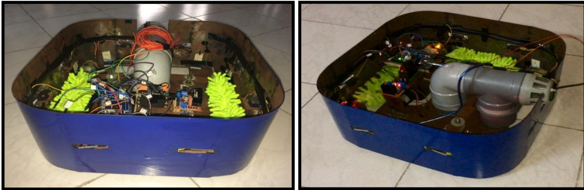
Figure 6: final assembly of the autonomous vacuum cleaning robot
