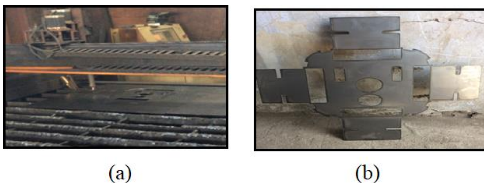
Figure 4: (a) Plasma cutting of chassis, (b) Final component after plasma cutting
