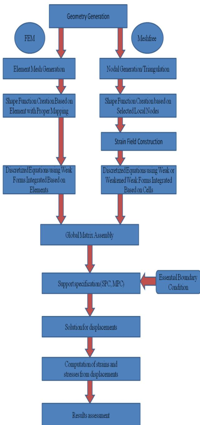
Figure 1.1 Basic Procedural difference in Grid based and Mesh free method:
