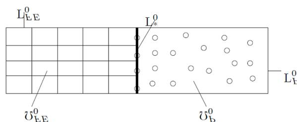
**Figure3.1 : Coupling of Particle and Finite Elements [78]**
