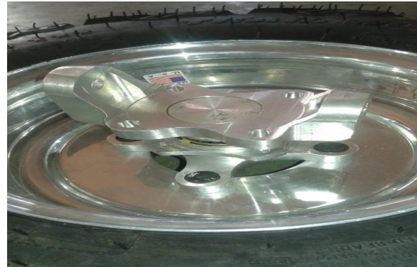
b> Knuckle joint attached to wheel
