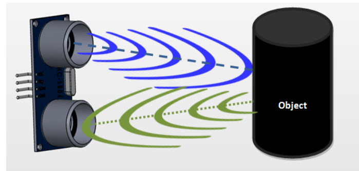
Fig 5. Working of ultrasonic sensor
