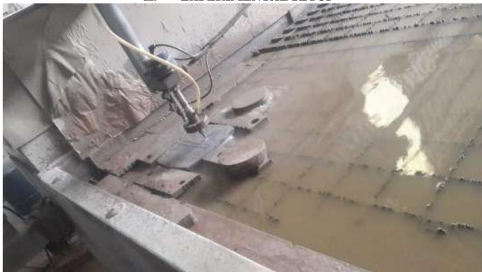
Figure 1 Abrasive water jet machining
