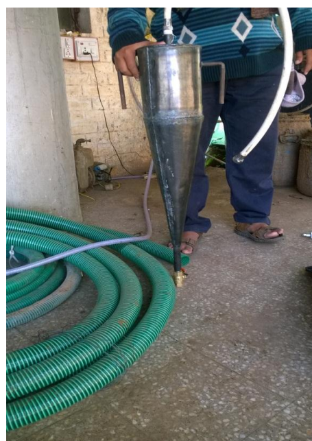
Fig 2 Cyclone Scrubbing Unit
