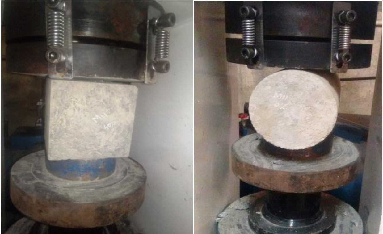
1. Cube and cylindrical specimens are subjected to compression and tensile test in the CTM
