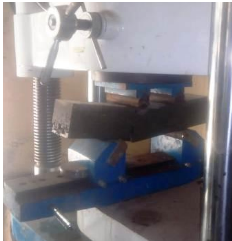
2. Beam specimens are allowed for flexural test in the UTM
