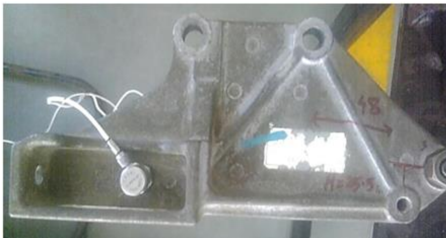
Figure V.2: bracket for modal analysis
