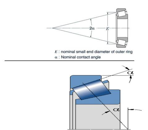
The axial load carrying capacity of tapered roller bearings increases with increasing contact angle  $\alpha$ .
