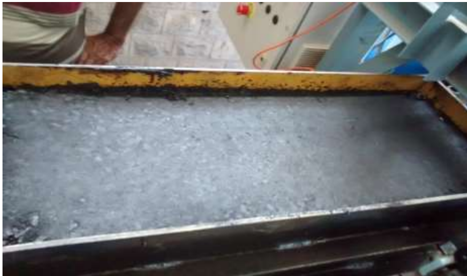
2. Before Rutting Test
