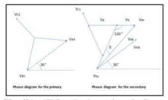
Where Vab and VAB are the primary and secondary line to line voltages respectively. To determine the turns ratio for the transformer, lets consider s triangle composed of VQ, Vby and Vab in the phasor diagrams, from which,
