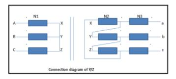
Fig.- shows a Y/Z phase-shifting transformer and its phasor diagram which shows that transformer can produce a phase-shifting angle ( $\delta$ ) defined by,
