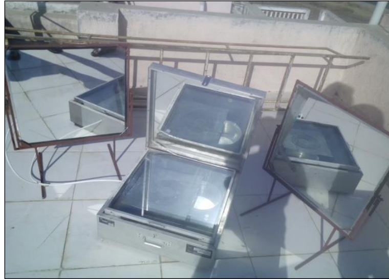
Figure 5. Actual Solar Water Pasteurizer Assembly
