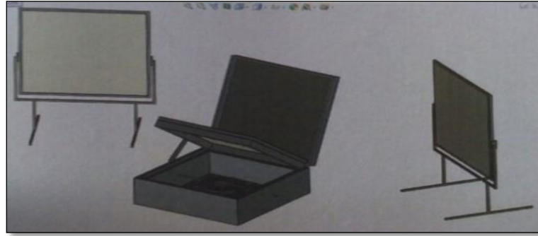
Figure 4. CAD Model of Solar Water Pasteurizer Assembly
