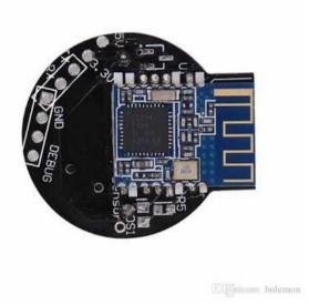
The above given figure is the iBeacon module Bluetooth base station 4.0 (Bluetooth Low Energy) near field localization.
