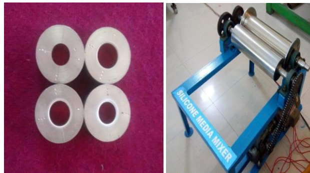
Fig 3.1: Copper specimens and Silicone media mixer
