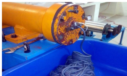
Fig 3.2: Extrusion honing process
