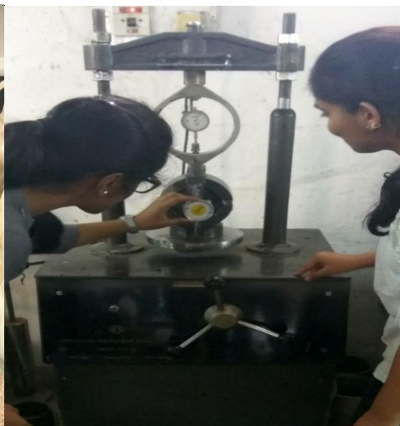
7. Marshall stability test
