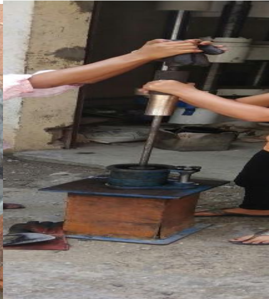
5. Prepration of Marshall Specimens
