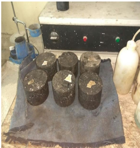
6. Casted Marshall Specimens
