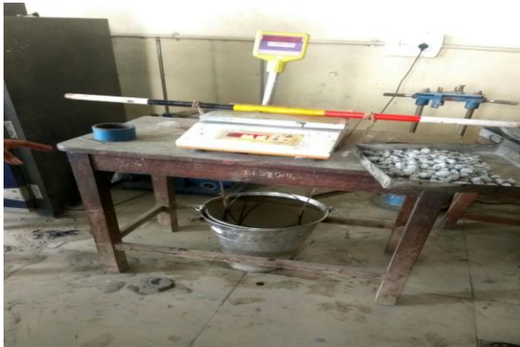
1. Specific Gravity Test Conducted For Aggregate
