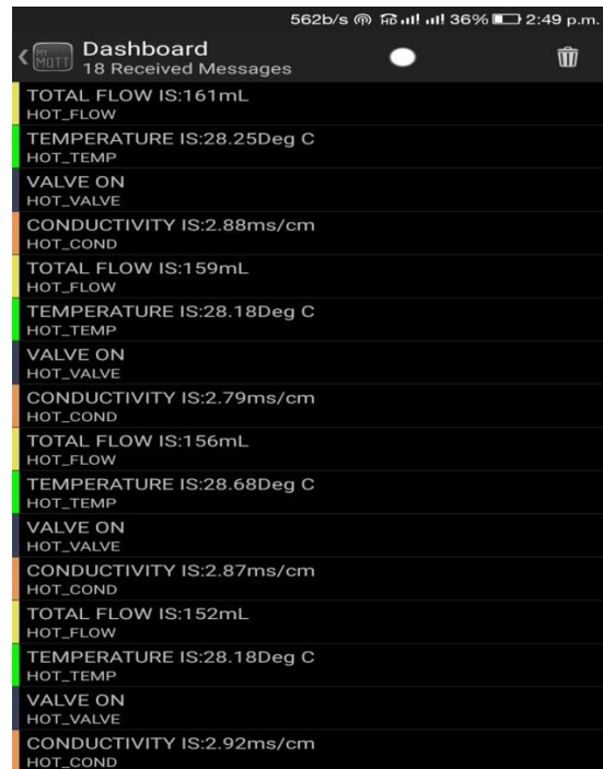
Figure 3.2. Data displaying on MQTT app
