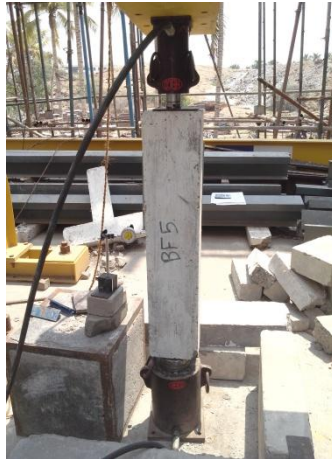
Figure 3.2 Testing of column specimen
