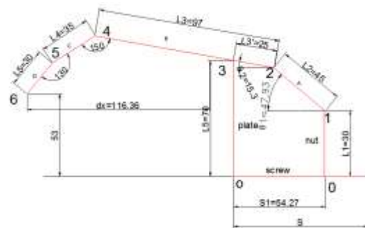
Figure 11: line diagram with parameter value when gripper is open
