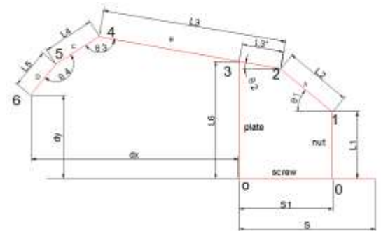
Figure 7: line diagram of one finger grasping model
