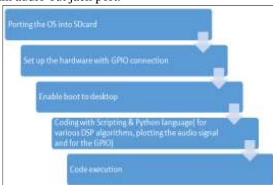
Fig 7 flow of the hardware set up
