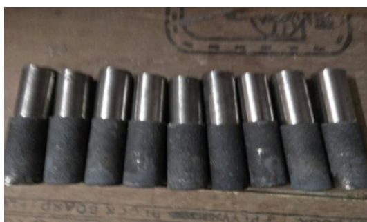
Cast iron Specimens after Machining
