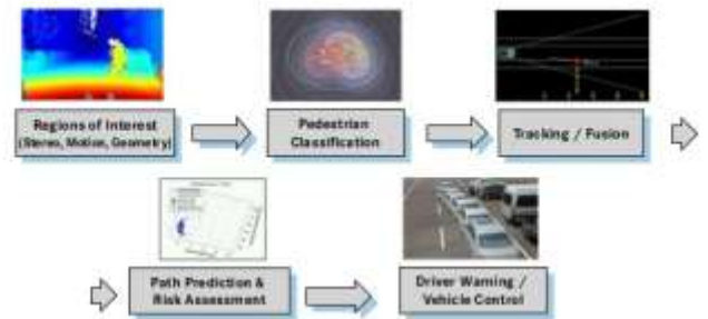
Figure 4.1: Logical Architecture for Pedestrian detection systems
