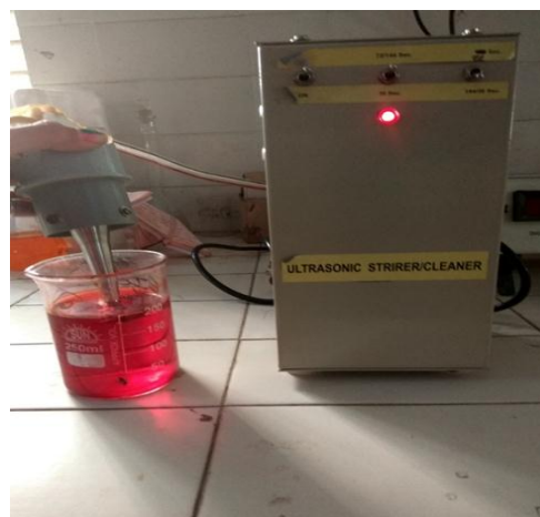
Figure 2. Ultrasonic Cavitation Apparatus
