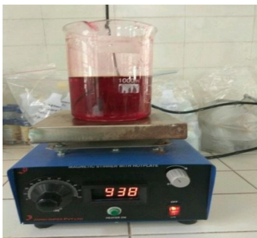
Figure 1. Adding \text{H}_2\text{O}_2 and \text{Fe}^{+2} in Raw Wastewater on Magnetic Stirrer
