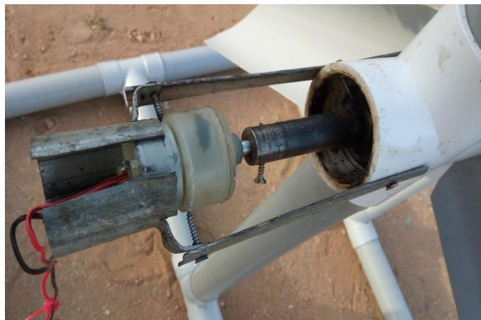
Fig. 7 Dynamo attached with shaft
