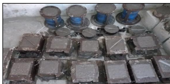
Fig: 1 casting of concrete
