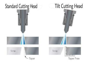
The effect of nozzle tilting angle on flow separation is by tilting the nozzle with an angle of 25 flow separation disappears inside the cut kerf. When the nozzle is tilted, the effect of impinging jet is much more significant. A
