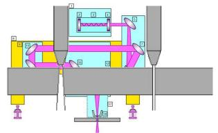
The focusing device consists of either a zinc-selenide lens or a parabolic mirror which brings the laser beam to a focus at a single point. Depending on the laser beam power, the focal length gives the distance of the focal point from the focusing optics.
