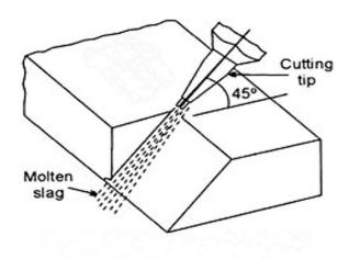
Kerf offset is traditionally adjusted by the machine operator. Prior to running a program, the operator must enter the kerf width so that the machine can calculate the actual tool path required to cut the part to the correct dimensions.
