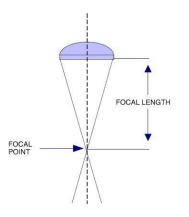
The focal point is positioned above, on or below the material surface according to the requirements of the material. The high power density results in rapid heating, melting and partial or complete vaporization of the material. The gas flowing from the cutting nozzle removes the molten mass from the kerf.
