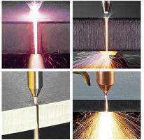
you program a 6" by 6" square, and the plasma arc removes 0.200" of material, as it cuts, then the resulting part is going to be 5.8" by 5.8". So the actual tool path has to be compensated by 0.100" to the side of the programmed path, all the way around the part.
