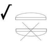
A dirty focusing lens heats up due to more intense absorption of the laser radiation and deforms. This leads to the focal position drifting towards the top.
