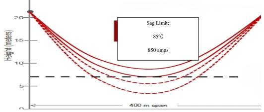
The above graph shows the general sag characteristics of a ACSR conductor.
