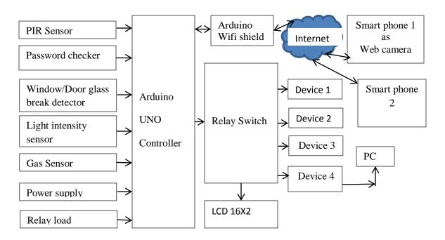
The PIR sensor is used to check the motion of intruder and if there is an intruder it sends the notification message to the house owner (smart phone 2) so that he can view the online recordings of web camera (smart phone 1). Here the old mobile phone is converted into web
