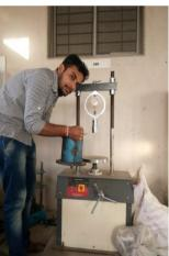
The Standard Proctor Test is carried out on the untreated soil samples as per IS: 2720-1980 (Part VII) and values of MDD and OMC were found out. The soil was treated with clayey soil and RBI Grade 81 for different proportions tested for soaked CBR value, MDD and OMC.
