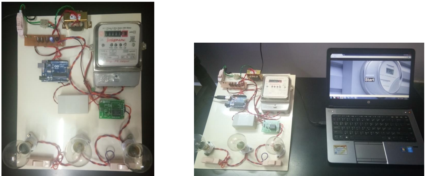
Fig 3.2 KIT setup for Smart meter
