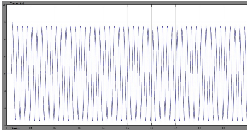
Figure 10. Current waveform after using series connected voltage source PWM converter.
