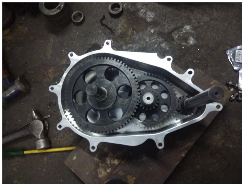
Figure 1: Open gearbox casing
