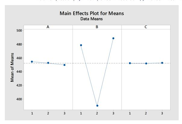
Main effects plot for UTS is shown in Fig. 9. The first plot displays effect of current on UTS using data means. The graph shows that the UTS decreases rapidly as current increases from 121 amp to 139 amp.
