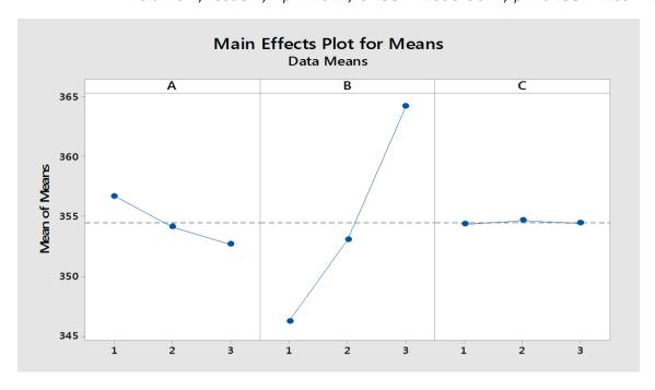
Main effects plot for hardness is shown in Fig. 6. The first plot displays effect of current on hardness using data means. The graph shows that the hardness decreases rapidly as current increases from 121 amp to 139 amp.
