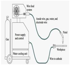
MIG welding is useful because you can use it to weld many different types of metals: carbon steel, stainless steel, aluminum, magnesium, copper, nickel, silicon bronze and other alloys.
