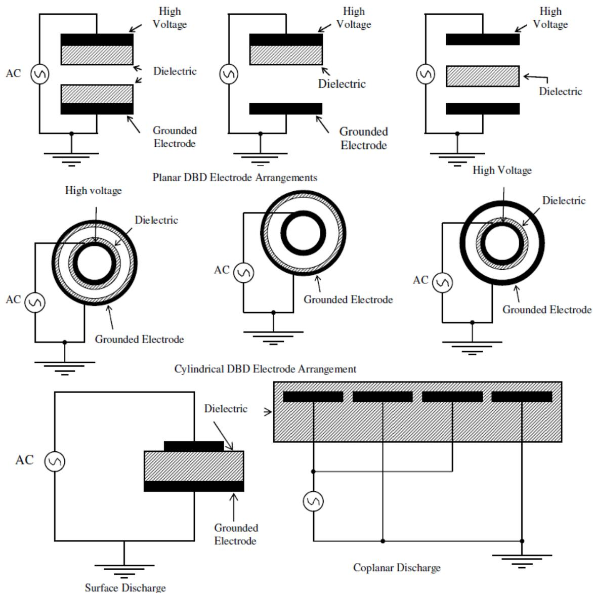
Fig. 1 Different arrangements of DBD
