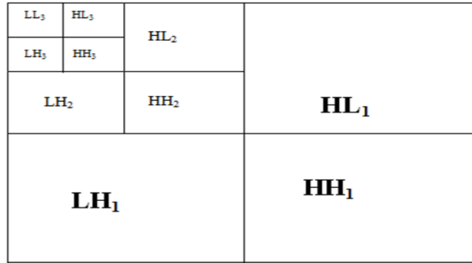
Fig 3: Three phase decomposition using DWT
