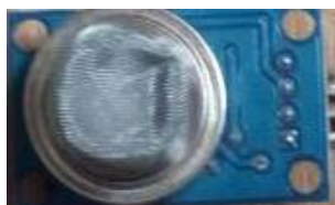
Fig-2: Gas Sensor
