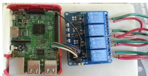
Fig. 3 Setting up the relay circuit for the Raspberry Pi.
