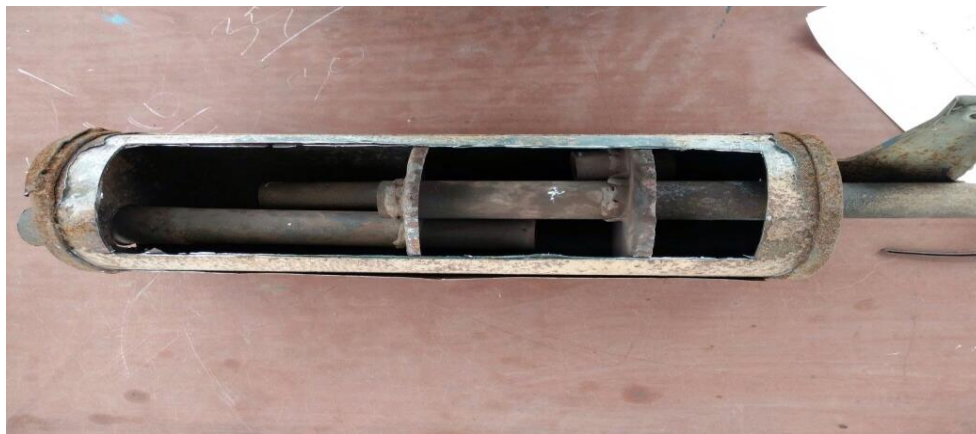
Figure 4 : Cut Section Of Scrap Muffler
