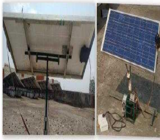
Fig. 3 solar panel with the solar tracking system.
