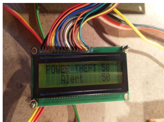
Figure 7.2.a LCD display with power theft alert
