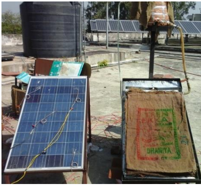
Fig.1: Photographic view of galvanized sheet arrangement with jute wick structures.
